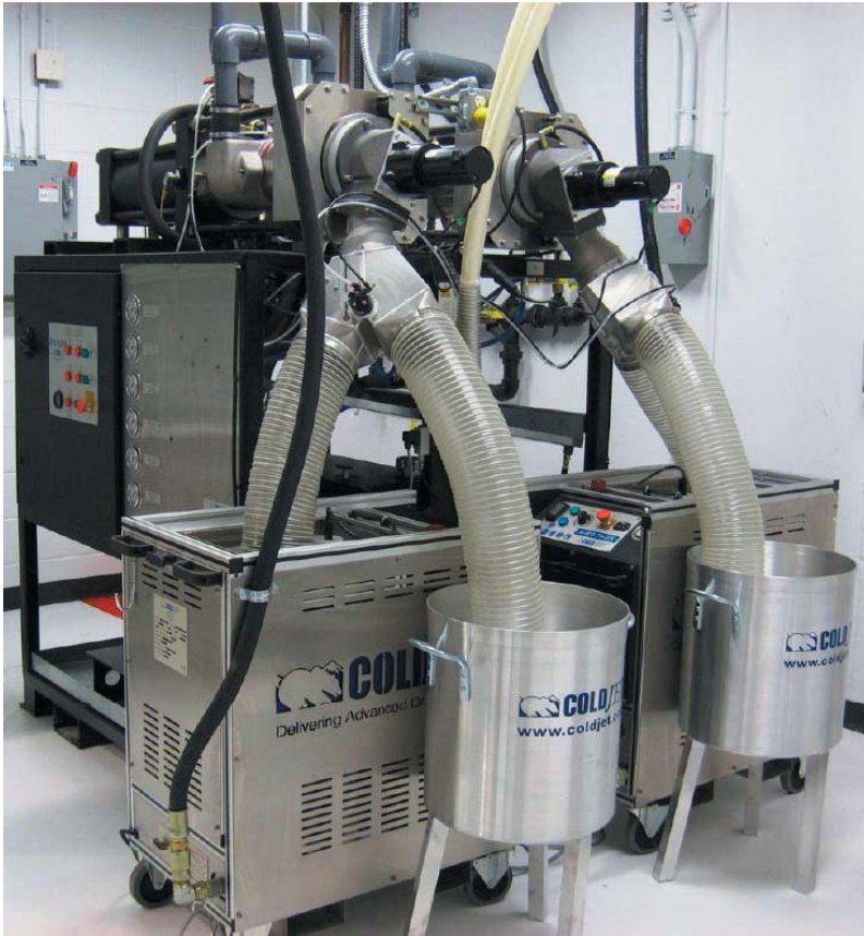
Left: P1500 equipped with two flow dividers and two pellet chopper assemblies (3 mm pellets only) providing a total of 4 dry ice pellet outlets.
